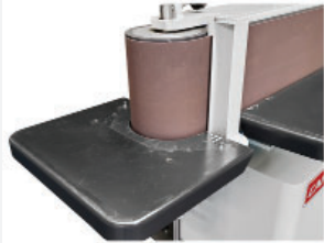
End table with hood removed for curve sanding. (tiltable to 45°)
