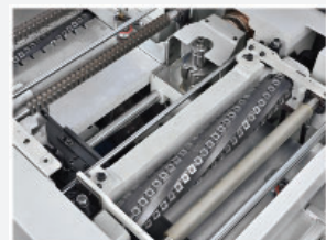
M412 with optional top and bottom spiral cutterheads installed
