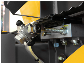
Blade spray mist lubrication system
