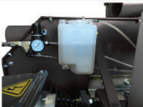
Blade lubrication system
