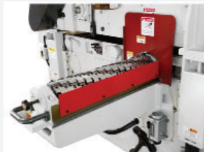
Removeable bottom spiral insert knife cutterhead
