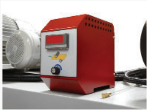
Inverter controlled variable planing speed
