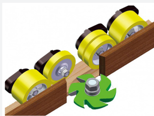
Various feeder wheel configurations to allow for blade and cutter clearance (DC40)
