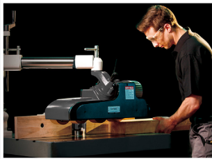
Power feeder operating on shaper
