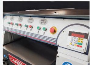
Operator controls with digital thickness control unit
