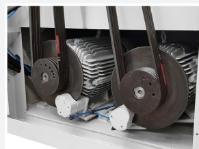
Pneumatic disc brakes for sanding heads
