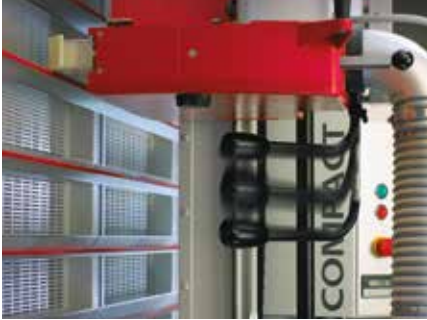
Saw unit with powerful motor (3.9 kW) and length-adjustable operating lever, which significantly facilitates plunging.
